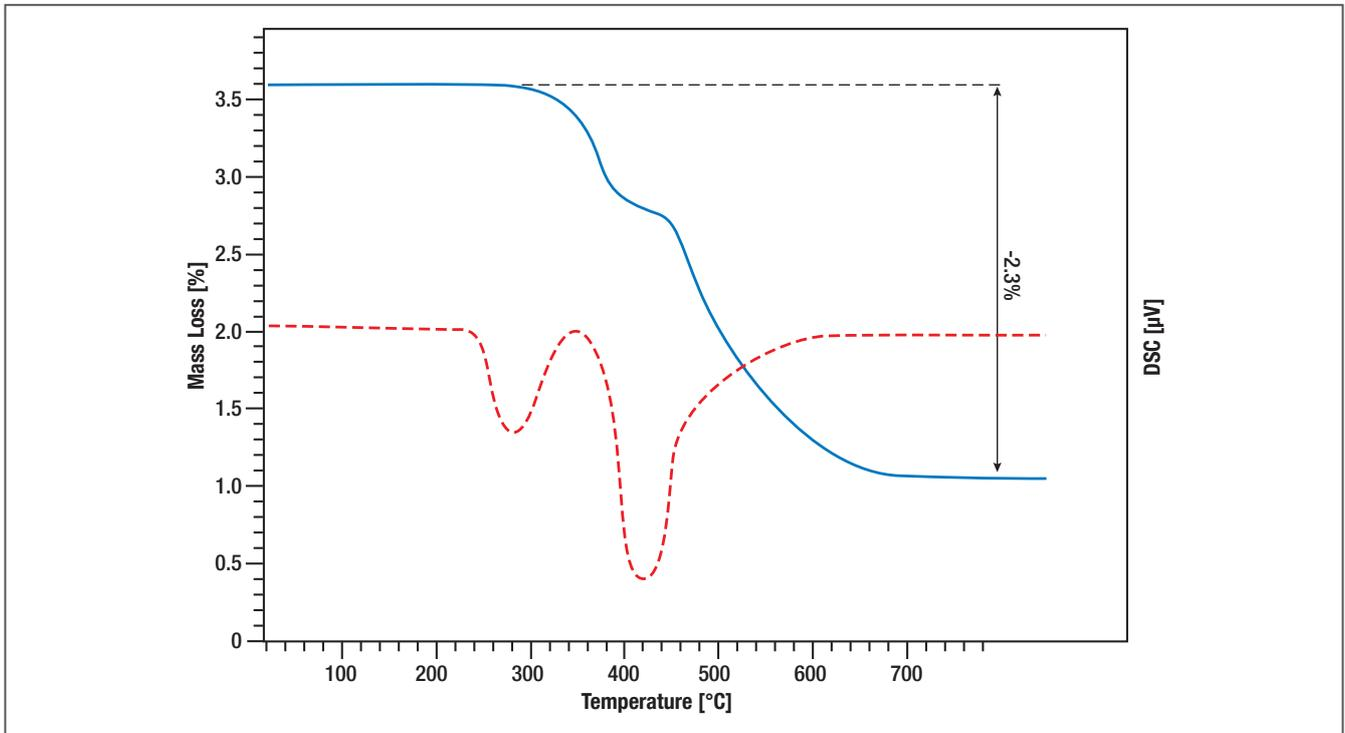
TG and DSC curves of TiH<sub>2</sub> in Argon at 10 K/min
