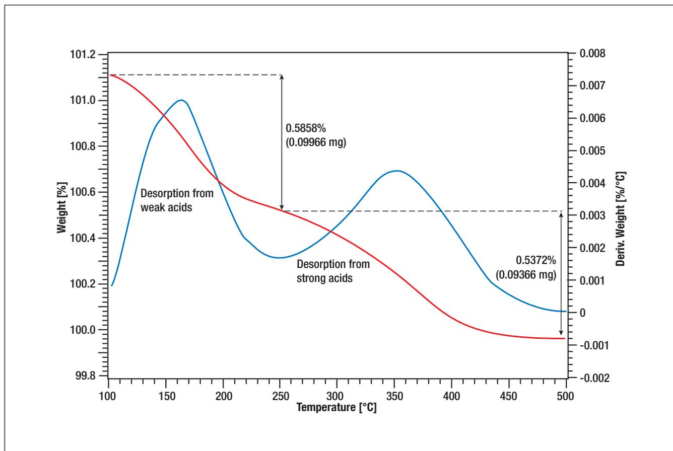
The distribution and relative strength of acid sites in zeolites are important indicators of its catalytic properties. The acidity of zeolites can be accurately measured with the temperature programmed desorption (TPD) of a base from the zeolite surface. The Linseis gravimetric Sorption Analyzers are useful tools for characterizing TPD, TPO or TPR profiles.
