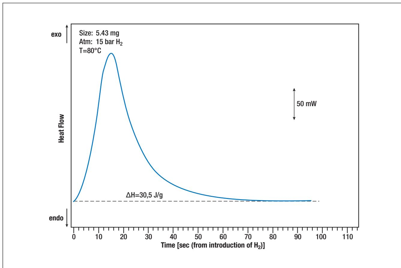
The measurement of sorption, oxidation or reduction heats of catalysts performed with volumetric methods are normally very time-consuming and need many hours. The LINSEIS Gravimetric Sorption Analyzer STA HP, which measures both weight change and DSC-signal, provides a much faster alternative. Within 15 minutes or less the sorption heats can be measured.
