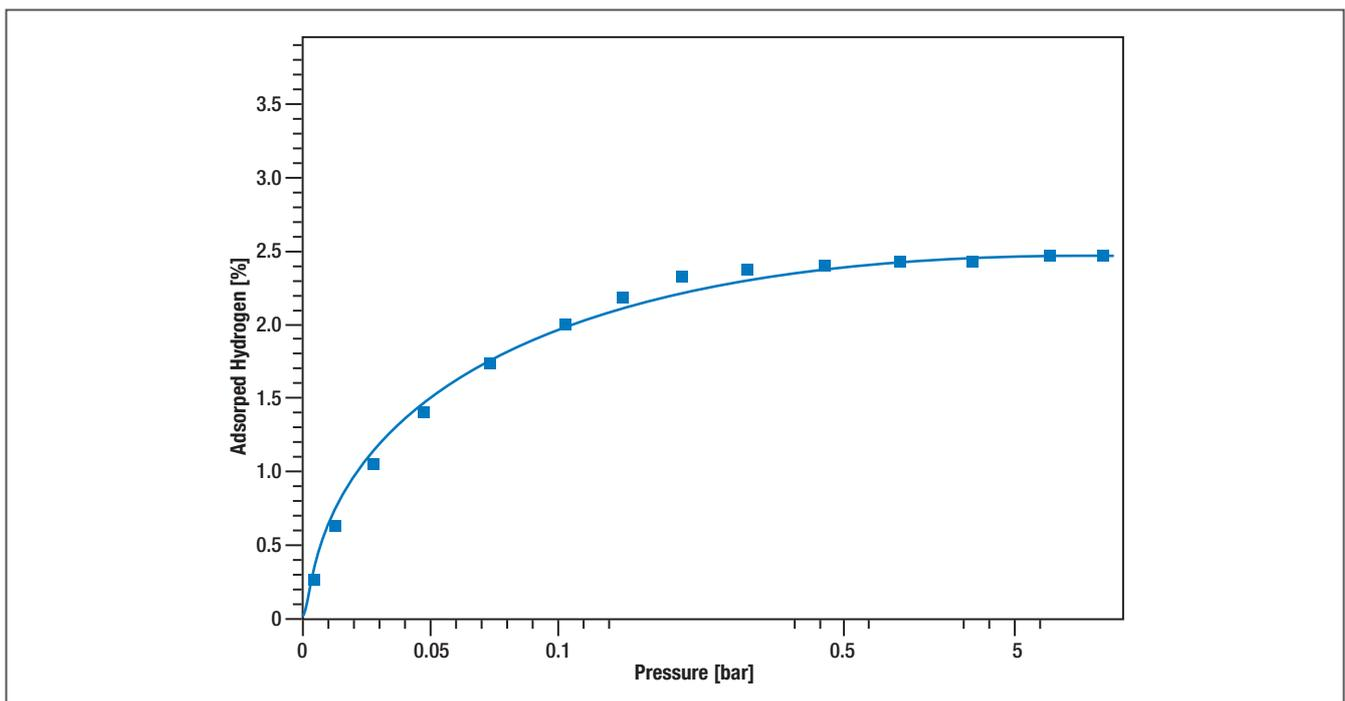
Adsorption Isotherm of Hydrogen on Titanium
