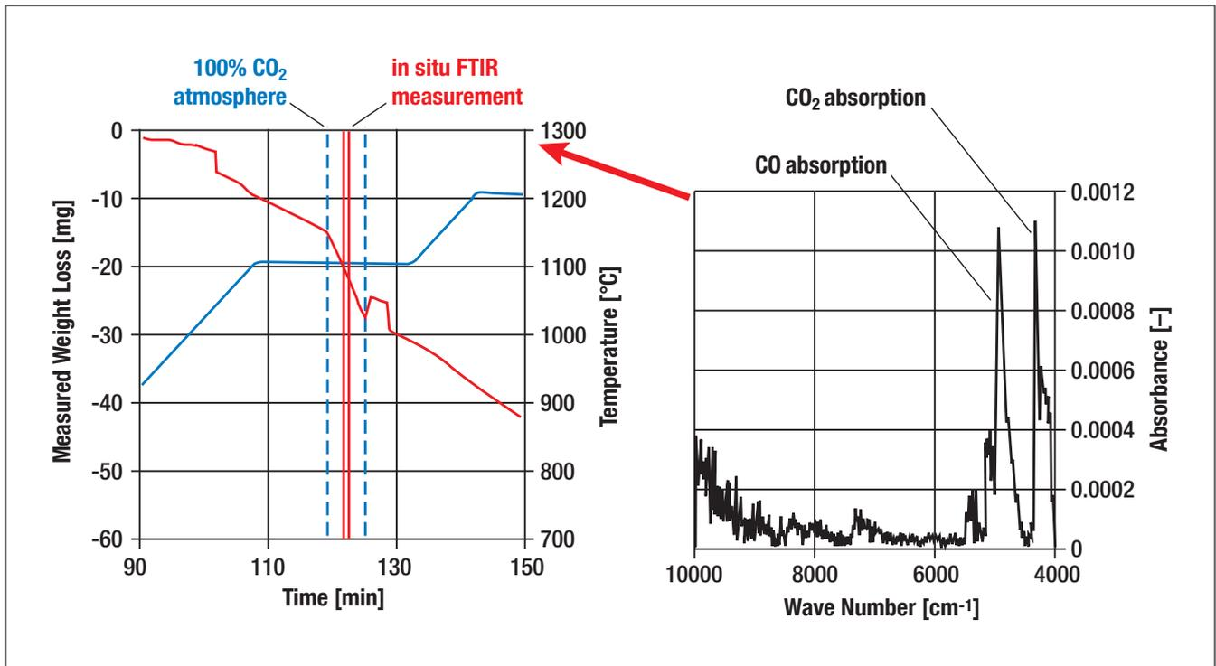
In-situ FTIR measurement during CO<sub>2</sub> gasification of an anthracite in a TGA system (sample temperature: 1100°C, pure CO<sub>2</sub> atmosphere [gas flow rate: 20 ml/min at 273 K, 0.013 bar] during FTIR measurement,
