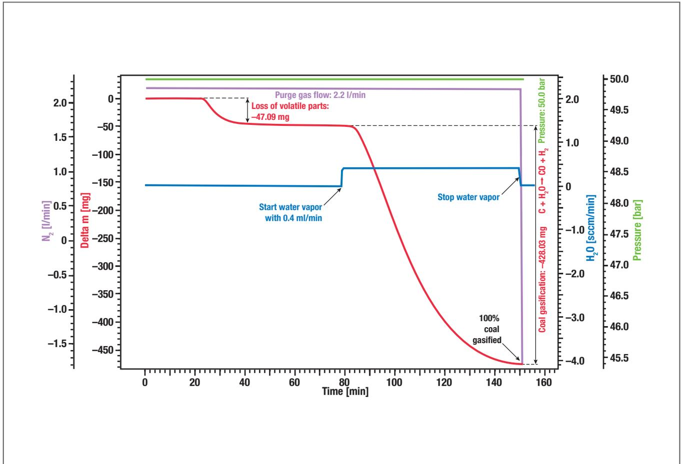
A common known application for HDSC measurements is the investigation of the so called coal gasification or hydro gasification. This process, where carbon is heated in a water steam atmosphere is used in some catalytical processes, for example to remove carbon monoxide (CO) from exhaust fumes and especially to get valuable organic compounds out from resources like charcoal or biomass.
