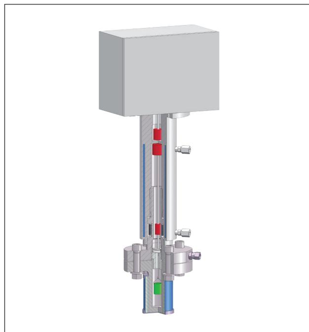
weighed. With the buoyancy of the sample the density will be calculated. With a compact construction of the magnetic suspension balance the density can be analysed in a large temperature and pressure range.
