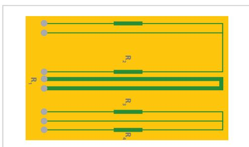
The LINSEIS Hot Point Sensors (HPS) work according to the transient plane method. They are suitable to measure small samples with dimensions down to 3x3x1 mm and to measure anisotropic samples. Due to the small amount of heat which is produced by the hot point sensors, they are a good choice to measure liquids with negligible convection.
